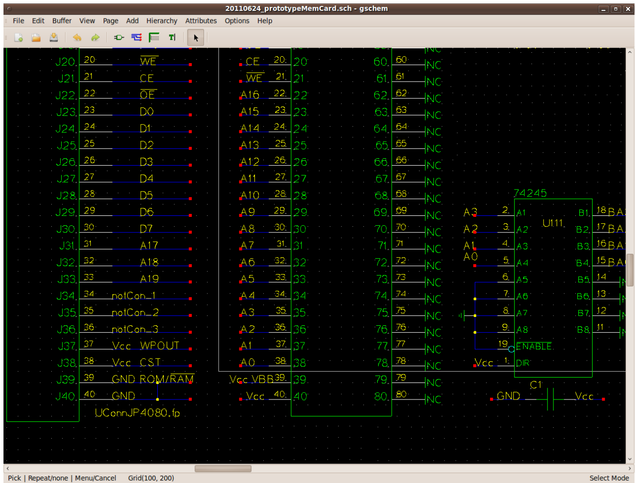
Lower left corner of schematic of memory card for prototyping.
